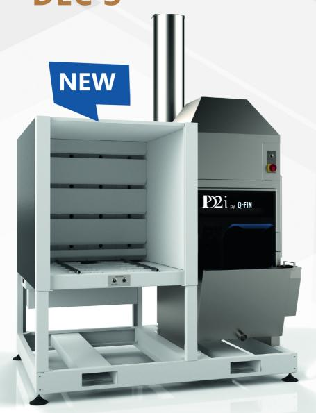
**DEC-3** is a self contained blow off station for cleaning tools, fixtures and turntables before and after the coating cycle. The dust is blown off via an air gun, then extracted by suction nozzles at the back wall and guided into a water based filtration and washing system.
